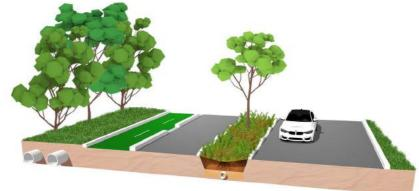
4: Duplicating the parallel stormwater pipe.
