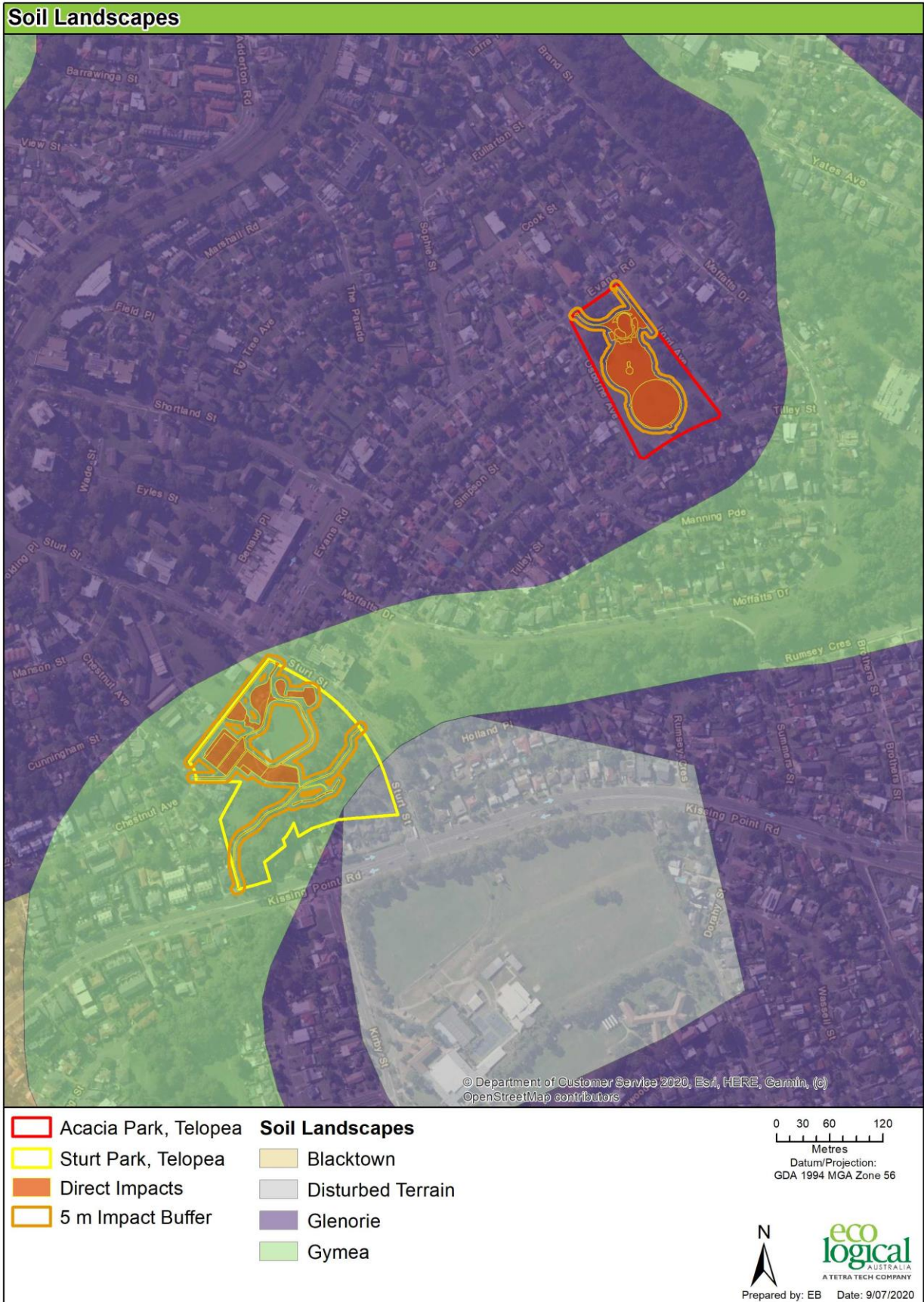
Figure 5: Mapped Soil Landscapes in relation to the study areas (Sydney 100k sheet)
