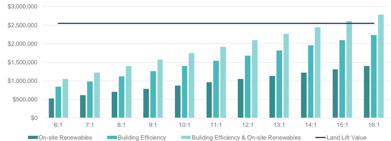
Figure 5: Land Lift Value compared to marginal cost of implementing the three sustainability pathways. While feasibility should be tested on a case-by-case basis, for this particular set of assumptions Land Lift Value is higher than all three pathways up to FSRs
