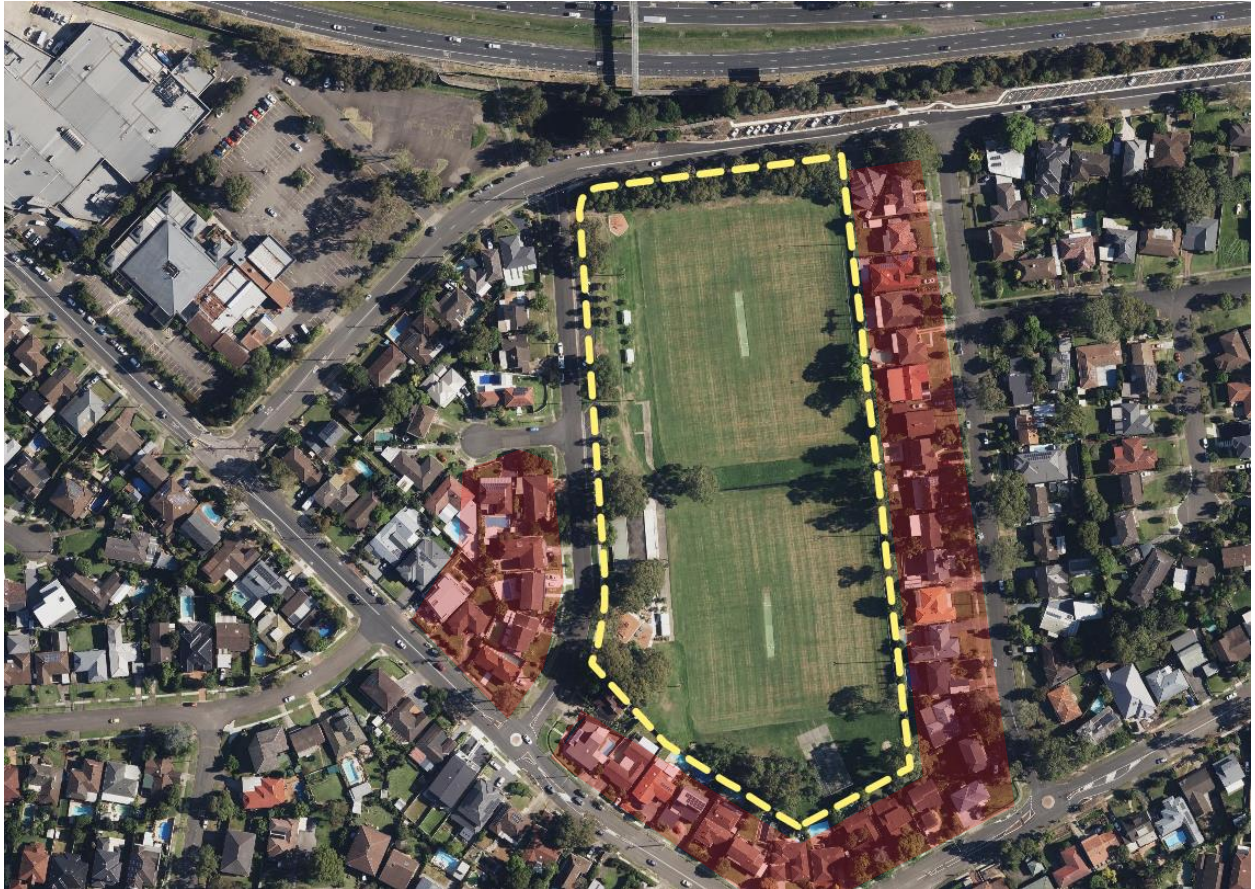
Figure 19 Location of sensitive noise receivers close to the limit of works, red = sensitive receiver (Source: NSW Planning Portal)
