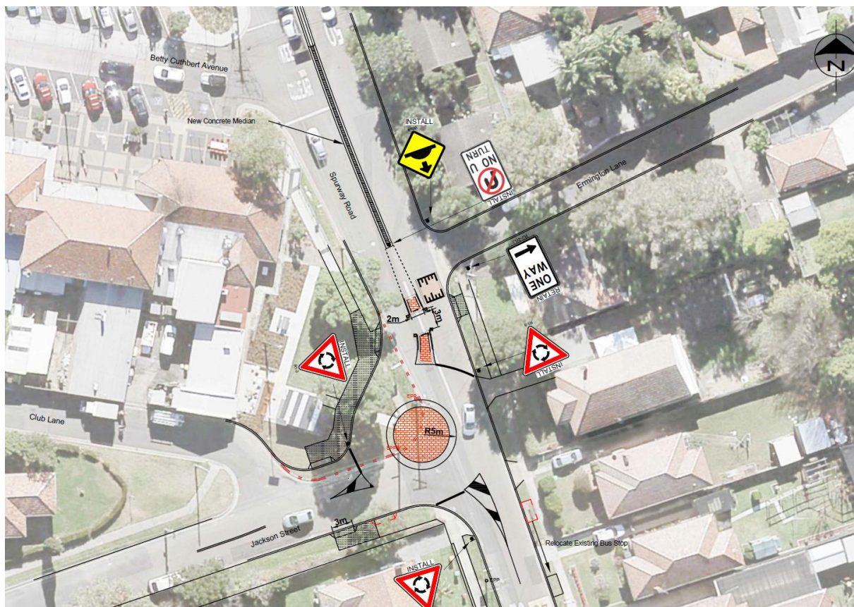
Figure 1: Concept plan showing the median island in Spurway Street at Betty Cuthbert Avenue and a roundabout at Jackson Street, Ermington
