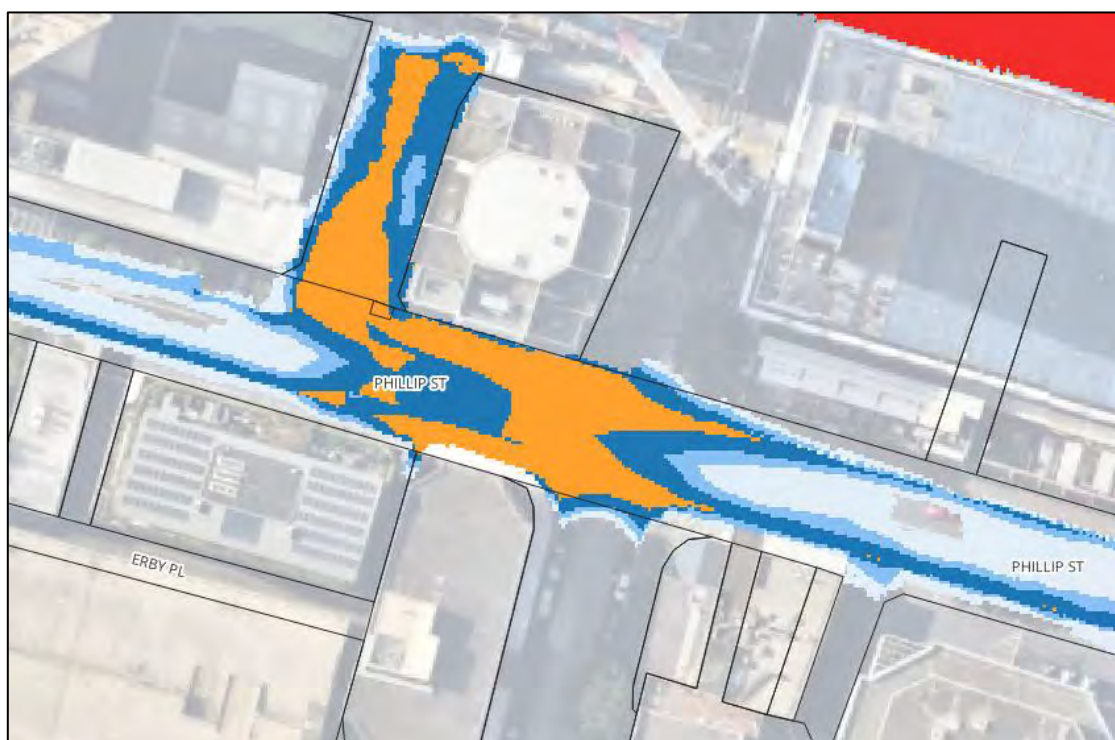
Figure 2-7: Base Scenario – Flood Depth for the 1% AEP Event, Peak River Level – Phillip Street
