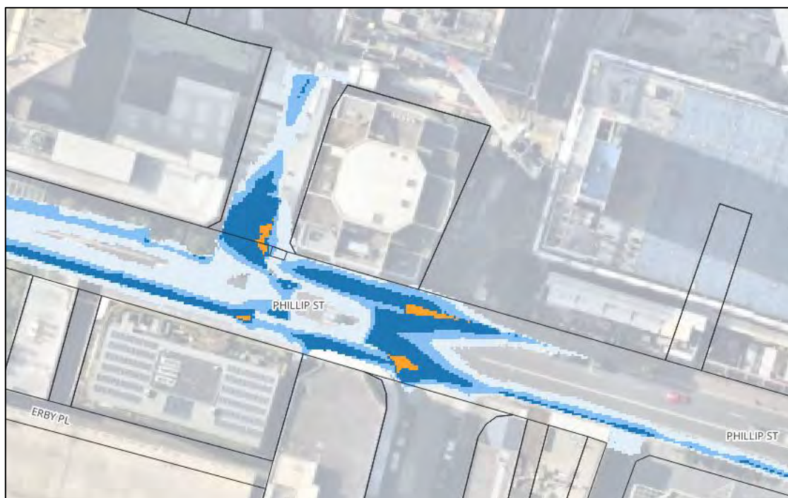
Figure 2-6: Base Scenario – Flood Depth for the 1% AEP Event, Low River Level – Phillip Street
