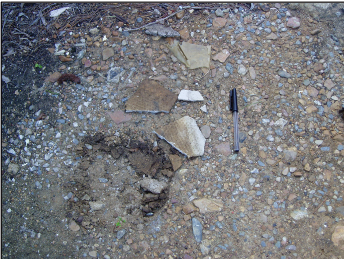
Image 4 Close up Example of Typical Asbestos Containing Fibre-cement Fragments with Dimples
