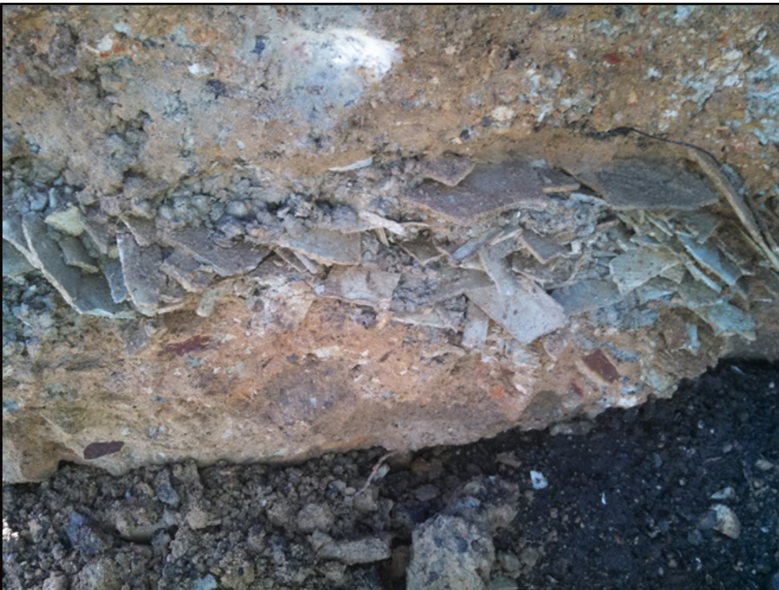
Image 2 Example of Bonded (non-friable) Asbestos Fibre-Cement Material
