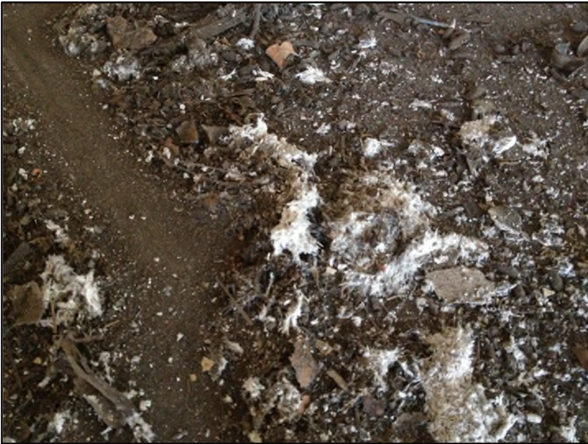
Image 3 Example of Friable Asbestos Lagging
